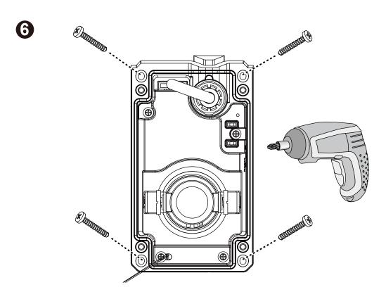
7. Install the top cover by fastening the anti-tamper screws.
