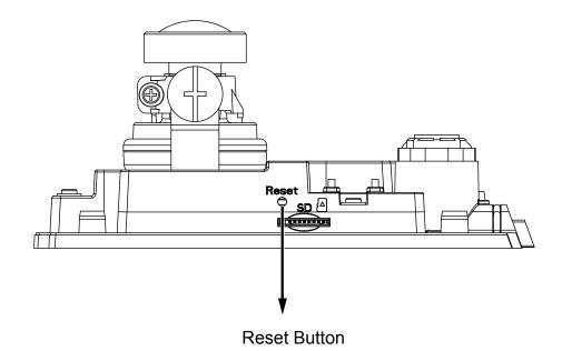
The reset button is used to reset the system or restore the factory default settings. Sometimes resetting the system can return the camera to normal operation. If the system problems remain after reset, restore the factory settings and install again.
