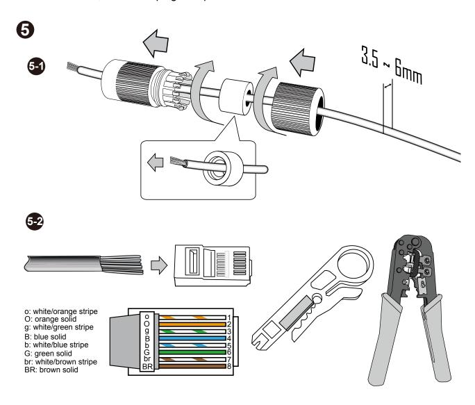
5-3. Route the cable through the cabling hole. Connect the Ethernet connector. Install the waterproof housing with a seal ring. Tighten up the connector.
